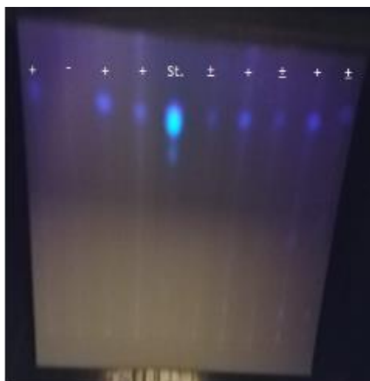
Figure 2: Thin layer chromatography results of feed samples were either negative (-), suspect ( \pm ), or positive (+) for AFs compared with standard (St.).
