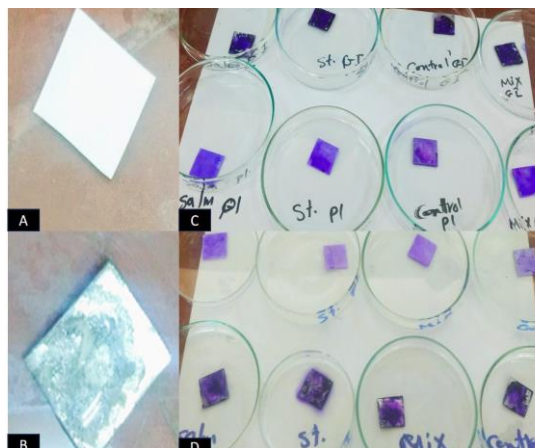
Fig. 1: The coupons were evaluated for biofilm growth and stained with 0.01% crystal violet. 1-A) Plastic coupon before biofilm development. 1-B) Galvanized steel coupon before biofilm development. 1-C) After six days of biofilm development, Staph. aureus and S. typhimurium form biofilms on plastic and galvanized steel coupons, either as mono-species or dual-species. 1-D) Plastic and galvanized steel coupons following biofilm formation by Staph. aureus and S. typhimurium , either as mono-species or dual-species, during 10 days of biofilm development.
