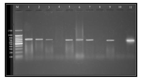
**Fig. 1:** Result of DNA amplification of *Br. melitensis* using Species-specific Primers electrophorized on (1.2 %) agarose gel. A single band of 731 bp in lanes (1, 2, 3, 5, 6, 7, 9, 11) indicates positive sample, while lanes (4, 8, 10) representing negative samples. Lane (M) indicates the DNA Ladder 100bp as DNA marker.
