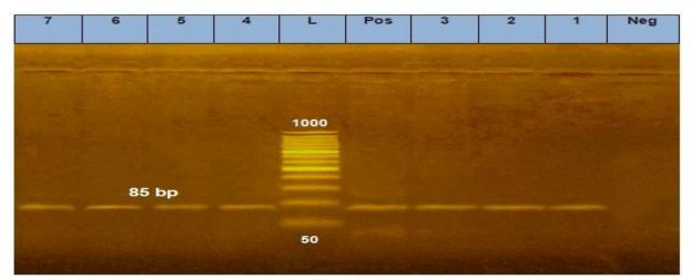
**Figure (6):** Agarose gel electrophoresis of PCR products for Salmonella isolates to detect *fim*A gene in genomic DNA. Lane L: gene ruler 50 bp DNA ladder. Neg: Negative control, Pos: Positive control. Lanes: 1 to 7 were positive samples.
